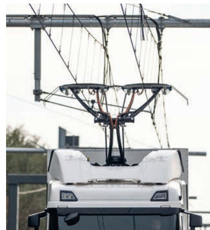
-Photos 1- ERS by overhead conduction (catenaries) - eHighway
