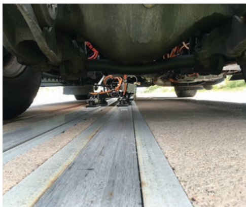
–Photos 4– APS rail grip tests on the test track of the Gustave Eiffel University in Nantes and winter tests in the Vosges.
