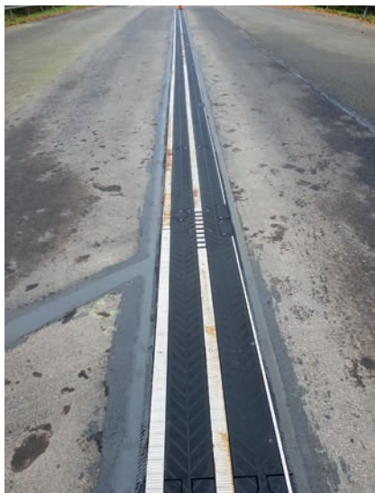
–Photos 4– APS rail grip tests on the test track of the Gustave Eiffel University in Nantes and winter tests in the Vosges.
