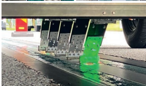
–Photos 6– Hollow rail ground conduction solution in Sweden.
