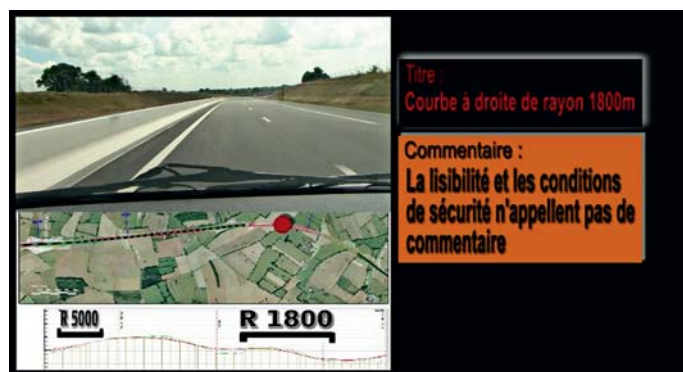
Photo 1 Description du matériel embarqué Description of onboard equipment
