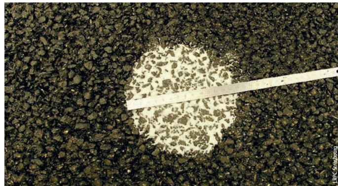
Photo 6 Mesure de la PMT Measurement of average texture depth
